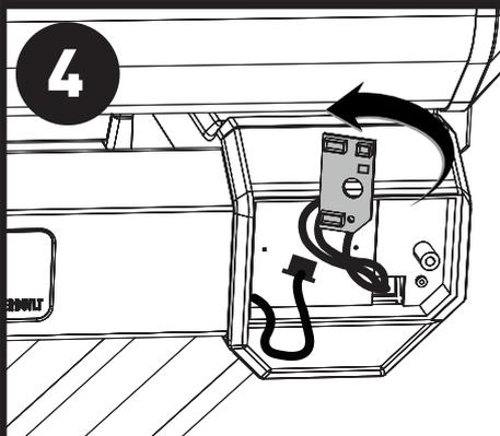
Disconnect 4 wires and carefully remove the PCB. There is adhesive tape on the backside of the PCB. Use caution.
