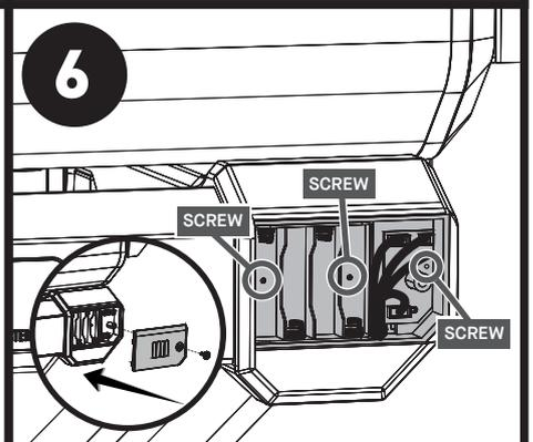
Use the screws to secure the new battery box and PCB. Replace the cover.
