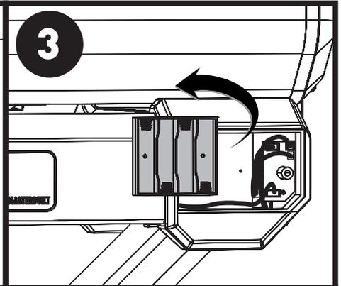
Disconnect and remove the battery box.
