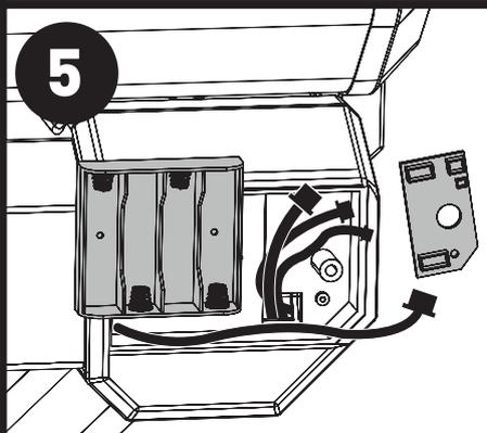
Connect the new battery box and PCB.
